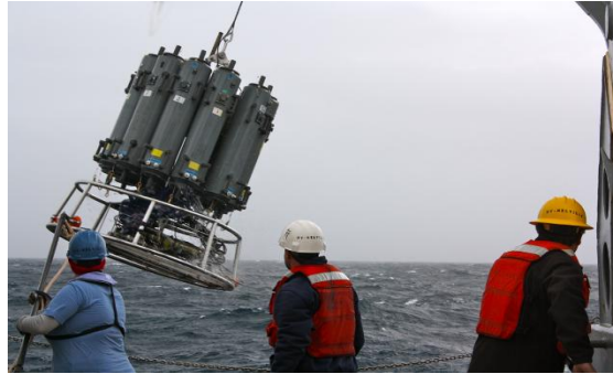
Figure 4: Oceanographers deploying a CTD; a device that's used to measure the Conductivity (salinity), Temperature and Depth of seawater. 4
