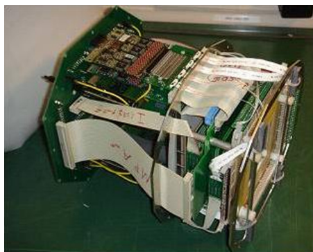
FIG. 3. Picture of SIMBA without its cylindrical coverage of 11.5 cm diameter.
