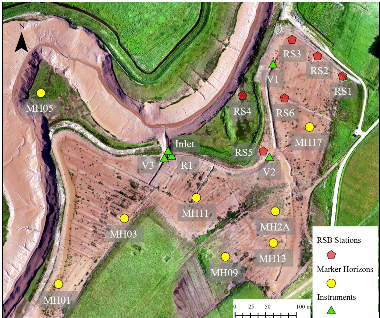
Figure 2.4. Converse deployment map with station legend. Orthomosaic created with imaging from a DJI Phantom 4 RTK Remotely Piloted Aircraft System (RPAS), piloted by Samantha Lewis on July 25, 2021, processed in Lewis (2022).
