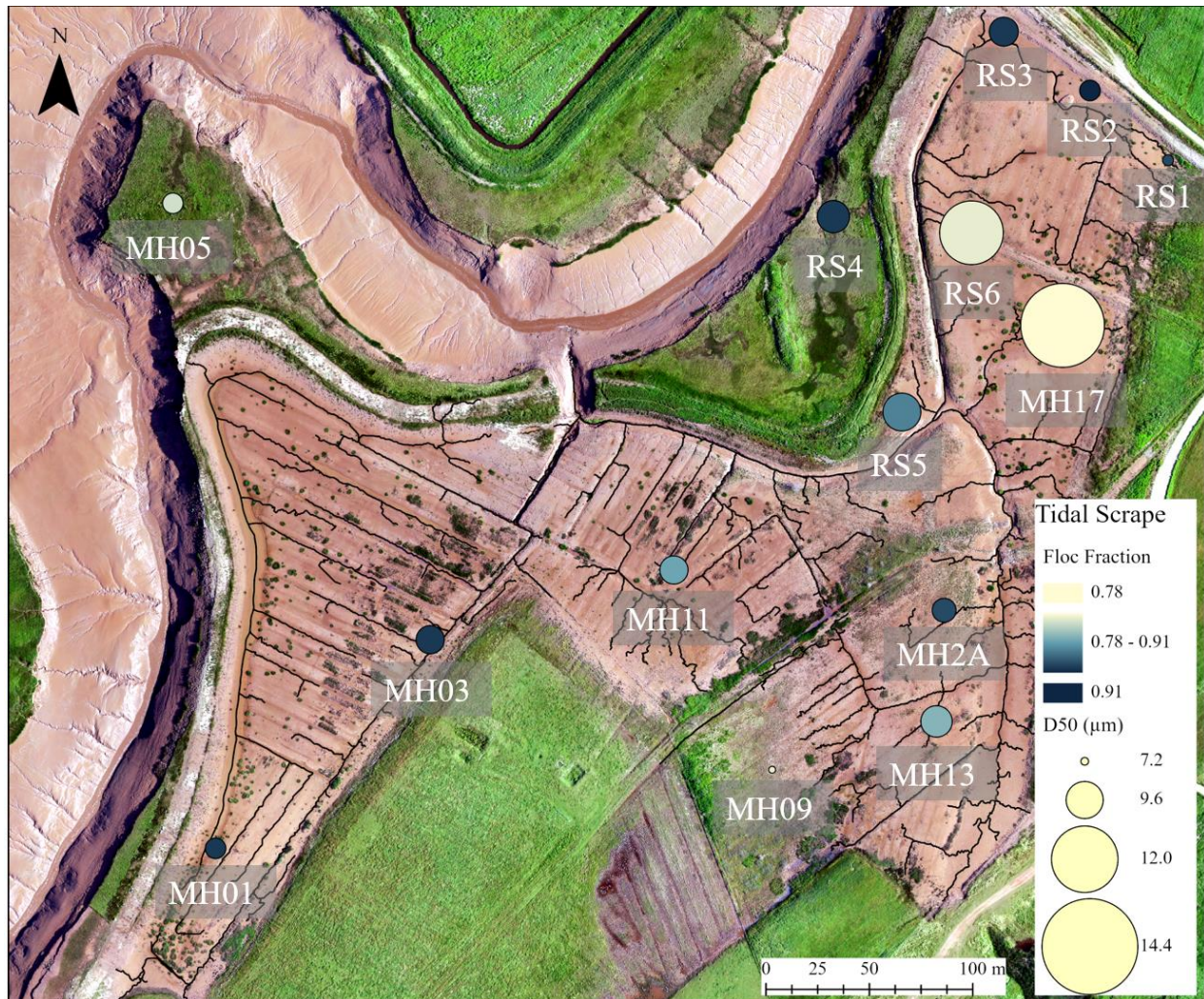
Figure 3.22. D50 ( \mu\text{m} ) and floc fraction averaged for all deployments. Orthomosaic created with imaging from a DJI Phantom 4 RTK RPAS, piloted by Samantha Lewis on July 25, 2021, processed in, with channel system shape from, Lewis (2022).
