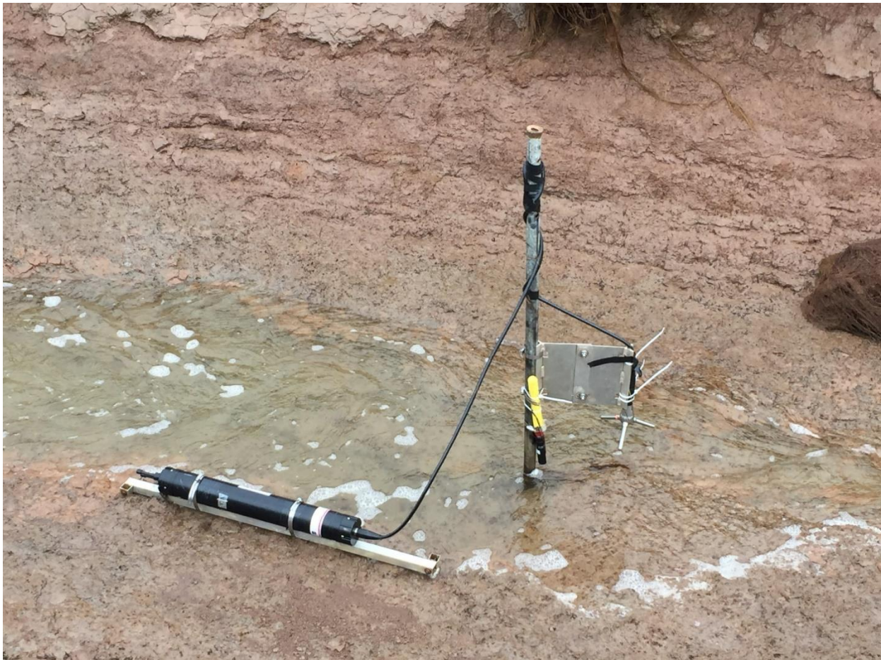
Figure 2.7. Acoustic doppler velocimeter (ADV) with RBR turbidity sensor setup in channel thalweg (station V3), taken August 21 st , 2020 (TransCoastal Adaptations, 2020).
