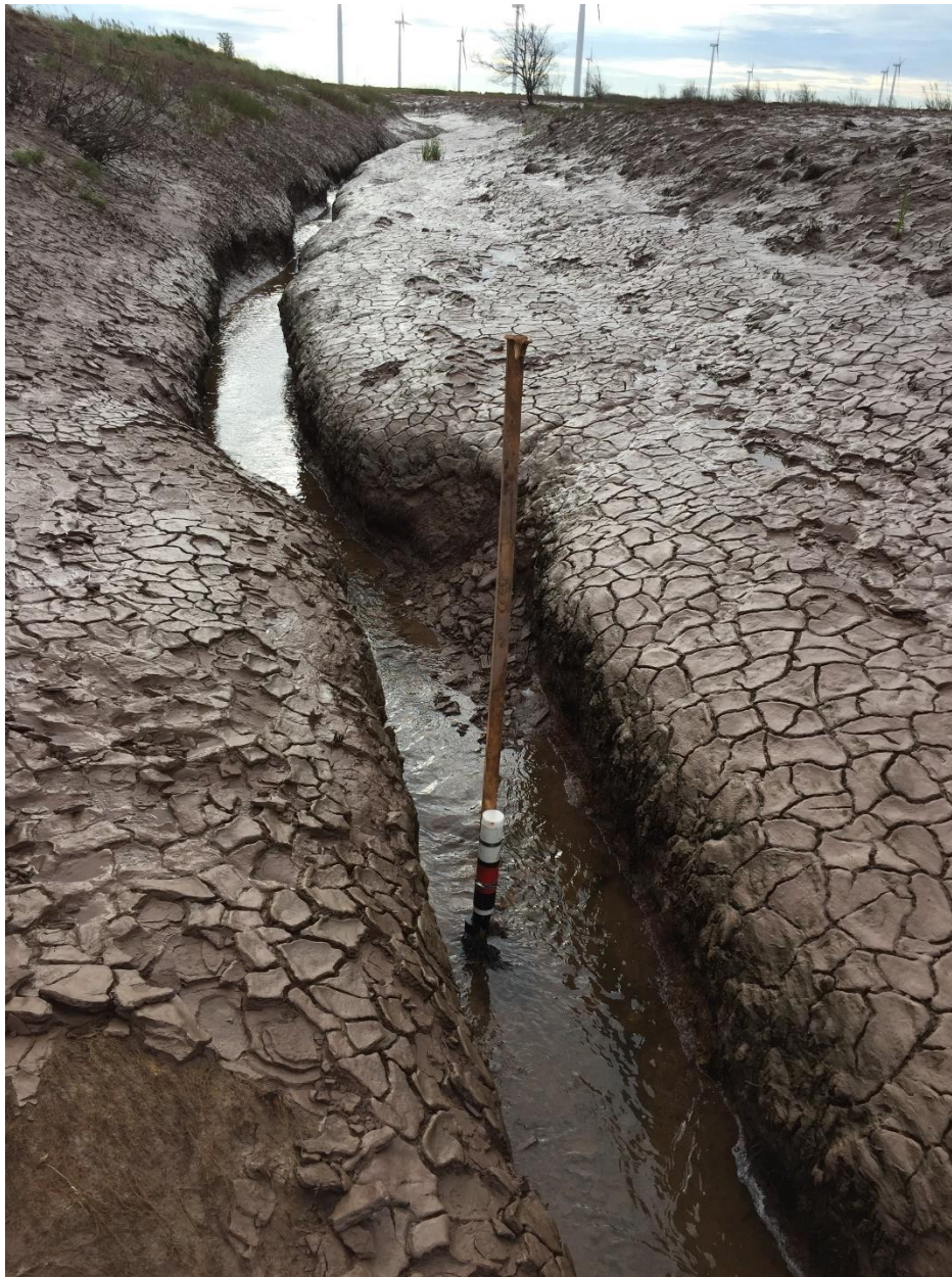
Figure 2.8. Ruskin XR-420 RBR turbidity sensor in thalweg of channel (R1 station), taken August 21 st , 2020 (TransCoastal Adaptations, 2020).
