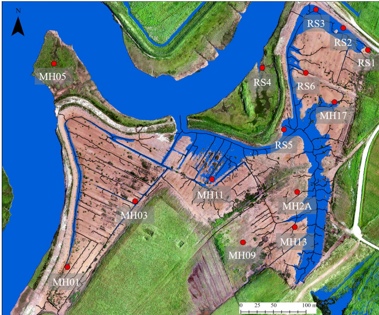
Figure 3.2. Site flooded to bankfull level (5.8 m CGVD2013). Orthomosaic and DEM for flood map created with imaging from a DJI Phantom 4 RTK Remotely Piloted Aircraft System (RPAS), piloted by Samantha Lewis on a) June 1, 2020, and b) July 25, 2021, processed in Lewis (2022).
