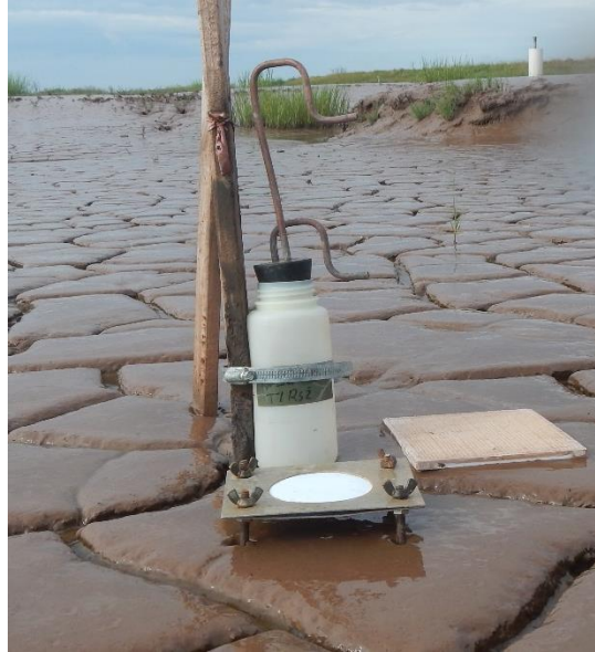
Figure 2.9. Sediment station (pre-collection) with sediment trap, tile, and rising stage bottle (RSB), taken July 23 rd , 2021 (TransCoastal Adaptations, 2020).
