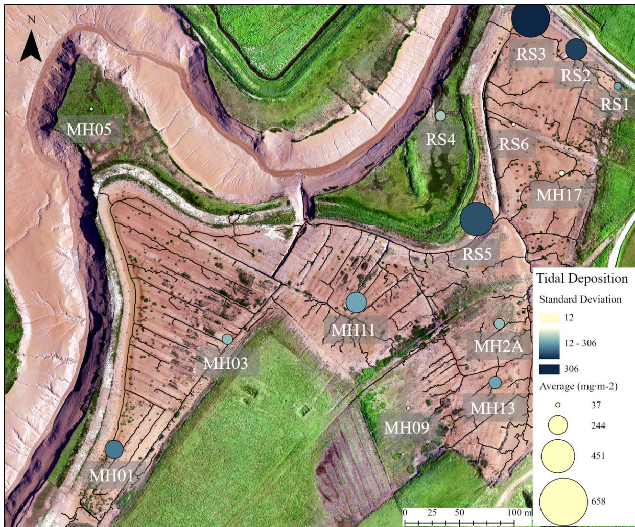
Figure 3.21. Average deposition in g\ m^{-2} and standard deviation for all deployments. Orthomosaic created with imaging from a DJI Phantom 4 RTK RPAS, piloted by Samantha Lewis on July 25, 2021, processed in, with channel system shape from, Lewis (2022).
