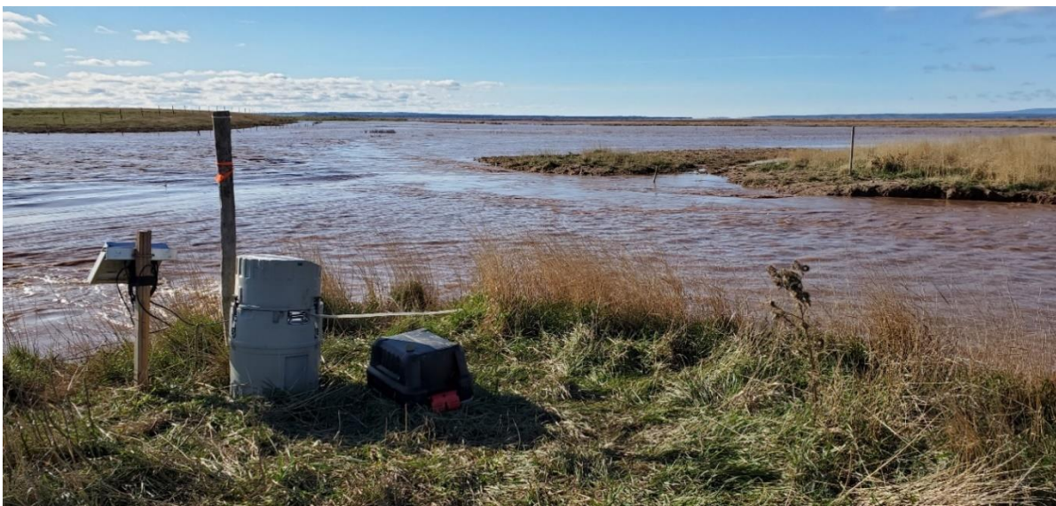
Figure 2.6. ISCO automated water sampler body setup on dyke beside inlet, taken November 15 th , 2020.
