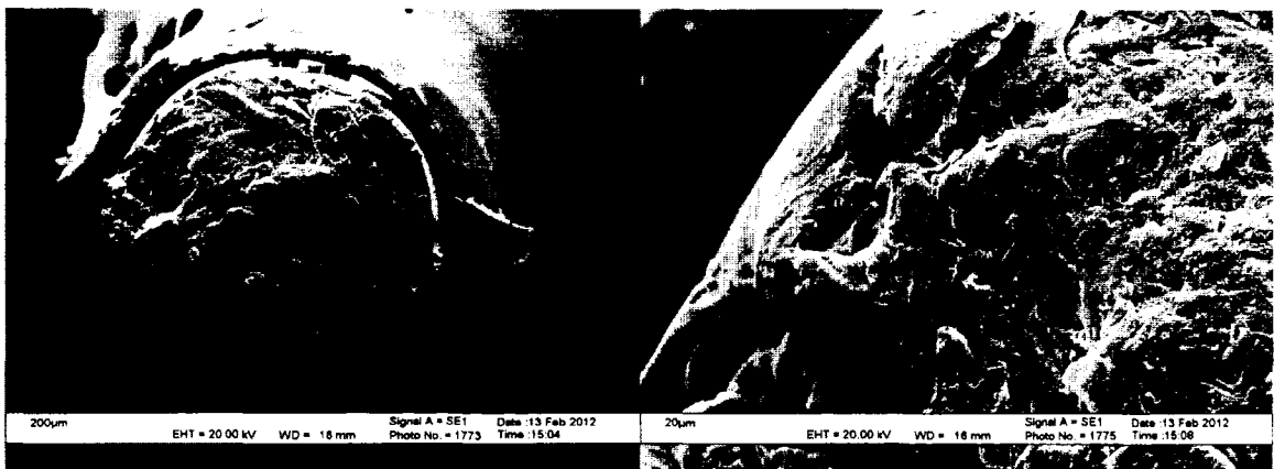
Figure 3.8: Fine Sandpaper Finish - SEM photographs of a 320 grit sanded scintillating fibre-end. The left panel shows the entire fibre face while the right panel is zoomed in. Note the PMMA cladding around the outside of the fibre in the right panel. Image parameters are reported on the photograph. The average granule size for 320 grit sandpaper is 36\text{ }\mu\text{m}
