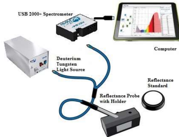
Figure 20. Fibre Optic Reflectance Spectroscopy system (Adapted from OceanOptics).
