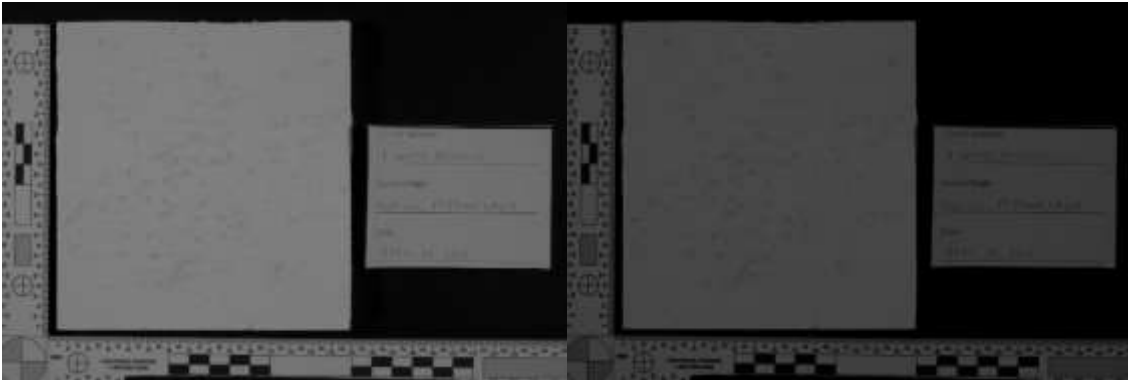
Figure 41. Example of Reflective Infrared Photography (Longpass Filter #87A) for the First Layer of Paint Stage (HDR White Acrylic 1 Left; Single White Acrylic 1 Right).
