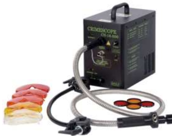
Figure 18. SPEX Crimescope with coloured filters and goggles (SPEX Forensics)
