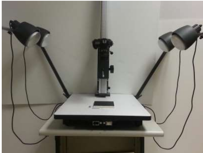
Figure 1. Copy-stand with tungsten light sources and mounted camera (example).
