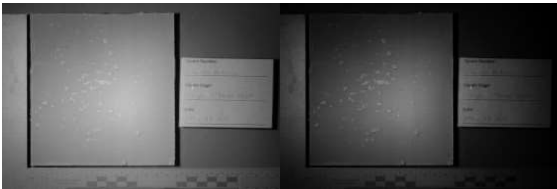
Figure 44. Example of Reflective Ultraviolet Photography for the First Layer of Paint Stage (HDR White Acrylic 1 Left; Single White Acrylic 1 Right).
