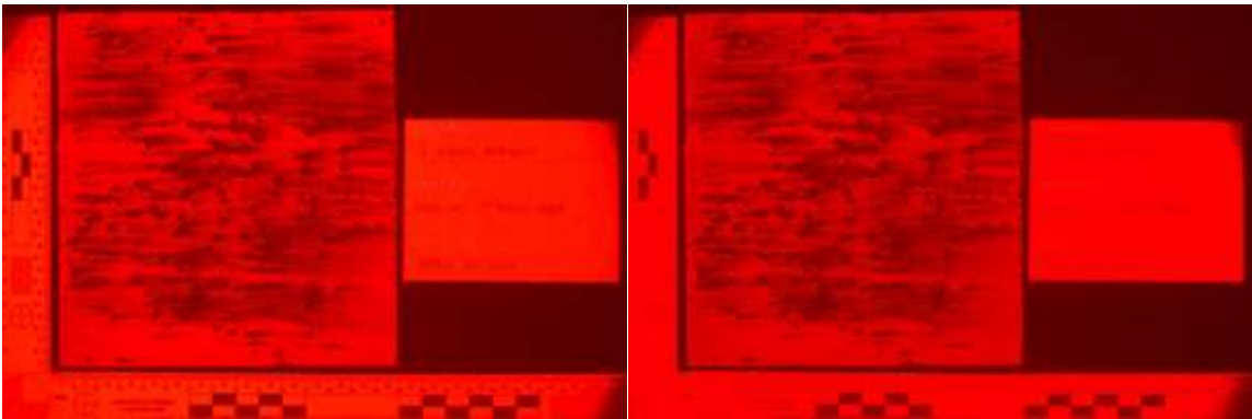
Figure 49. Example of Fluorescence Photography (Red Filter 575 nm) for the Bloodstain Pattern Stage (HDR White Acrylic 1 Left; Single White Acrylic 1 Right).
