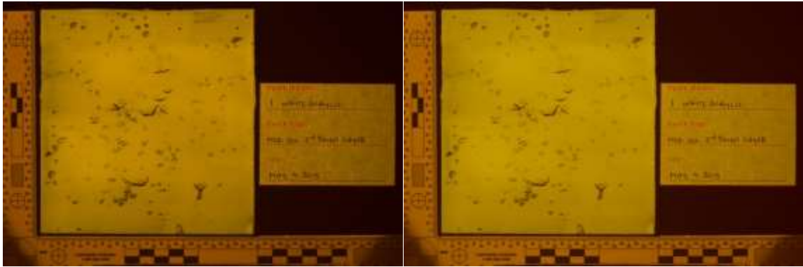
Figure 51. Example of Fluorescence Photography (Yellow Filter 445 nm) for the Second Layer of Paint Stage (HDR White Acrylic 1 Left; Single White Acrylic 1 Right).
