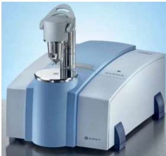
Figure 21. Attenuated Total Reflection Fourier Transform Infrared Spectrometer (Bruker Optics).
