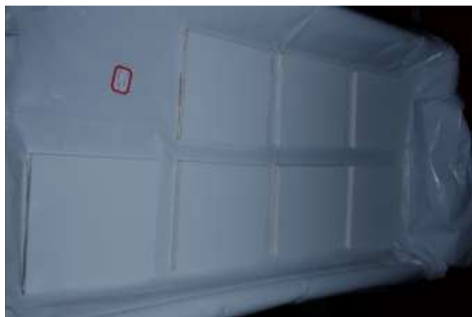
Drying cart with painted drywall squares.
