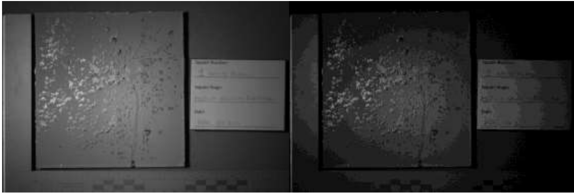
Figure 43. Example of Reflective Ultraviolet Photography for the Bloodstain Pattern Stage (HDR White Acrylic 1 Left; Single White Acrylic 1 Right).
