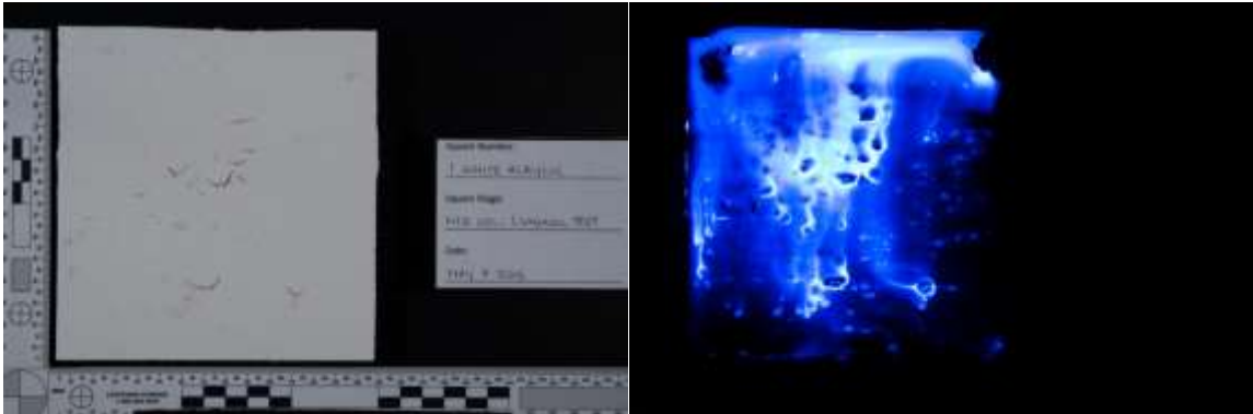
Figure 37. Example of Standard Photography (Luminol testing) for the Second Layer of Paint Stage (White Acrylic 1)
