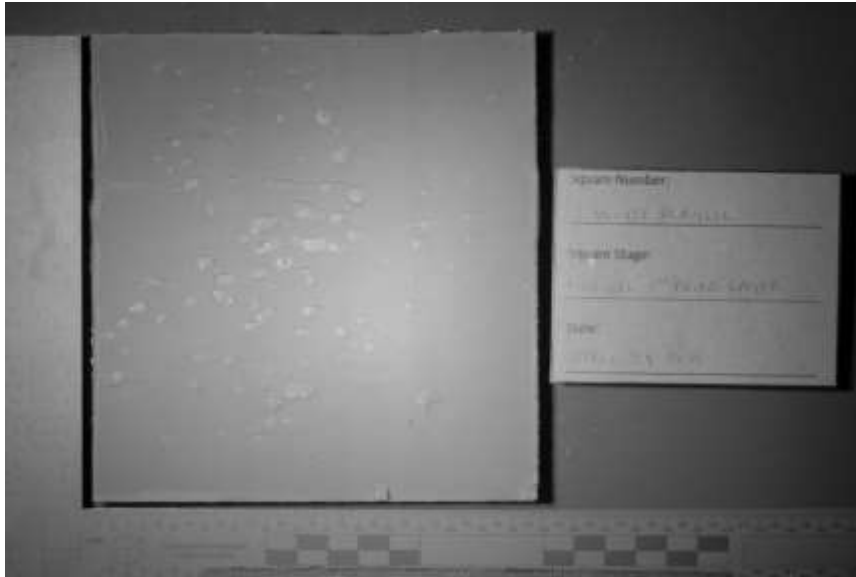
Figure 29. Example of Reflective Ultraviolet Photography for the First Layer of Paint Stage (HDR White Acrylic 1)
