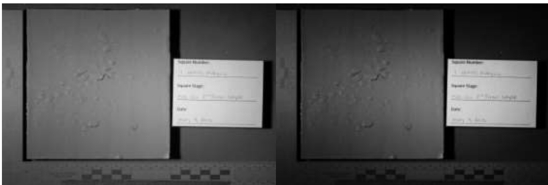
Figure 45. Example of Reflective Ultraviolet Photography for the Second Layer of Paint Stage (HDR White Acrylic 1 Left; Single White Acrylic 1 Right).
