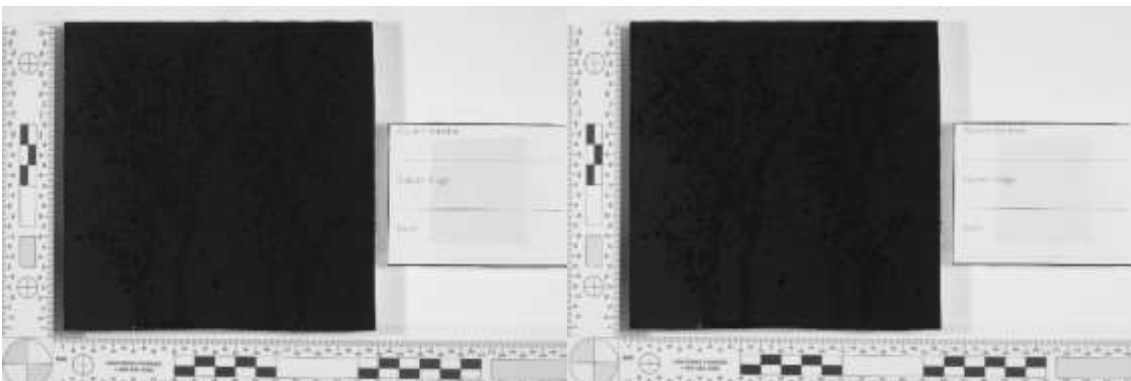
Figure 40. Example of Reflective Infrared Photography (Longpass Filter #87A) for the Bloodstain Pattern Stage (HDR Black Latex 9 Left; Single Black Latex 9 Right).
