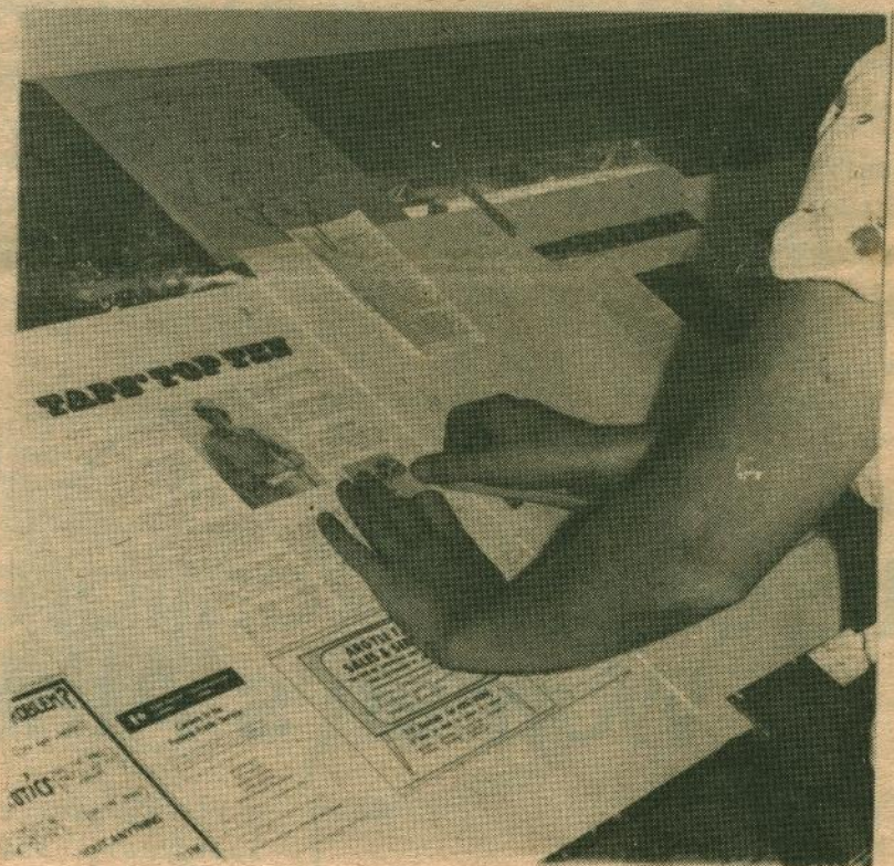
The type-set copy is now in the 'paste-up' stage where the columns are waxed and 'pasted' on tabloid-size sheets.
