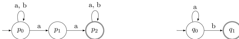
(a) NFA P accepting all words with the substring aa (b) NFA Q accepting all words of the form (a^*b)
