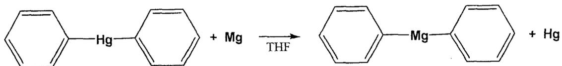
**Scheme 2.4.1: An obsolete preparation for diorganomagnesium reagents from diorganomercury reagents.**<sup>128</sup>
