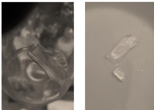
Figure A4: Large, “block-like” crystal of 6 , in the bottom of a 20 mL screw-cap vial (left), and in a weight-boat (right). The image on the left has been recoloured to “grayscale” for visual clarity.
