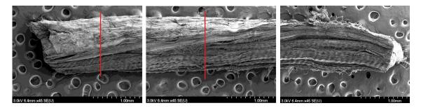
Figure 4.9: A representative panoramic scan of one of the tendon samples that was later scanned under high magnification. The red lines show both cross-sections where the scans were done.
