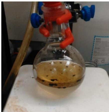
Figure 9: Reaction flask of Sat. KOH Solution and PTC.
