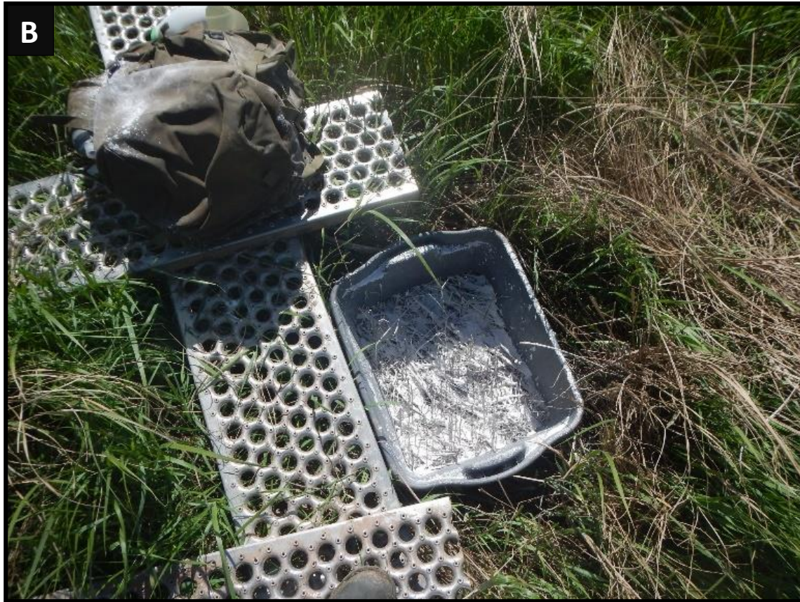
Figure 6. Example of rod surface elevation table measuring technique (a) and (b) and marker horizon initial set-up. Photos taken June 4, 2018 at Belcher Street salt marsh.
