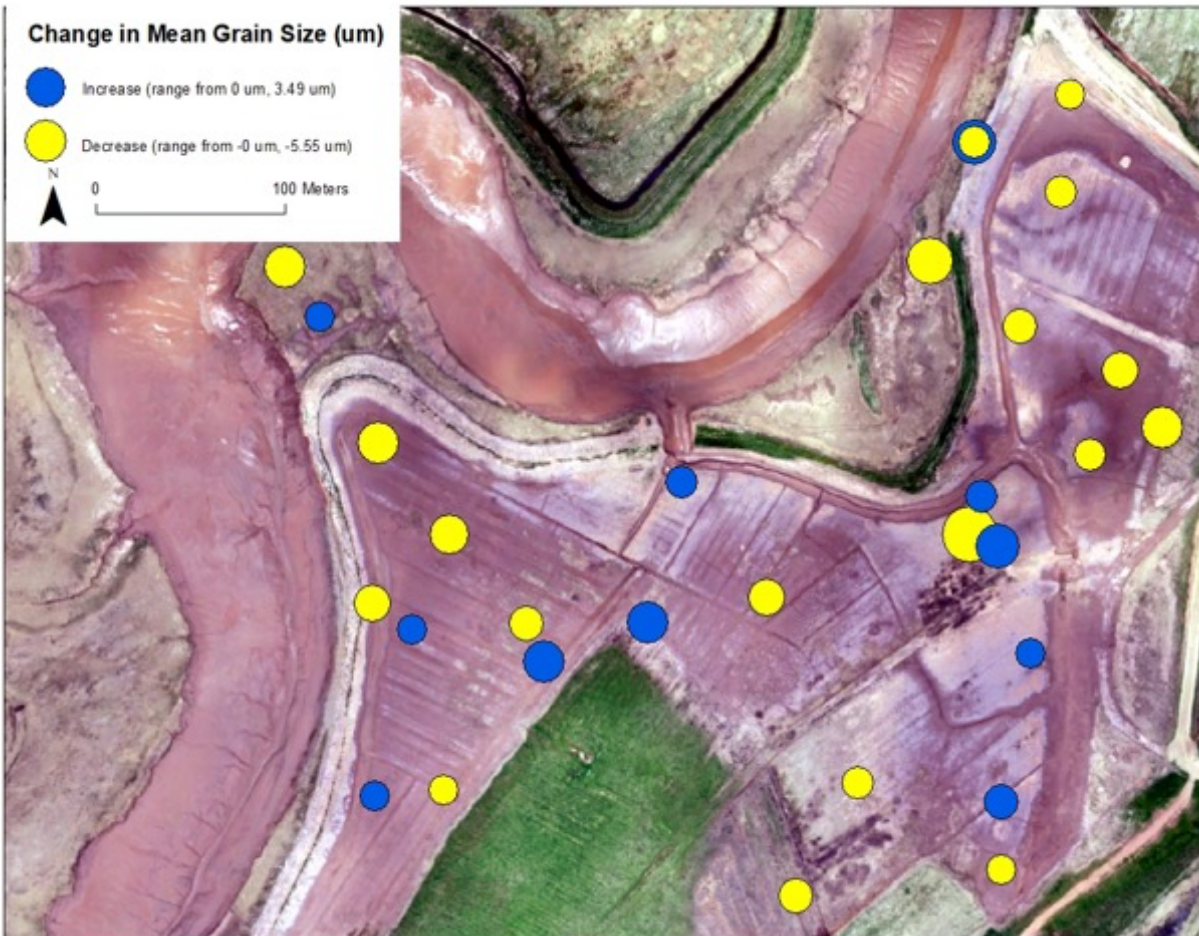
Figure 4.15. Change in Mean Grain Size ( \mu\text{m} ) from August to November at the Converse Marsh. Orthomosaic generated from low altitude aerial imagery collected by a DJI Phantom 4 RPAS, piloted by Samantha Lewis on 2020/06/01.
