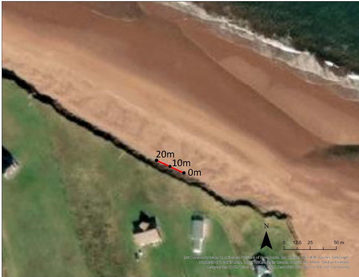
Figure 3.2. Example of a 20m transect. Sub-transects measured at 0m, 10m, and 20m.
