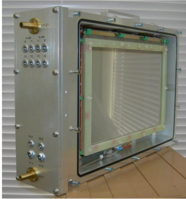
Figure 3.6: Photograph of the Double PPAC detector after removing its window plate [112].
