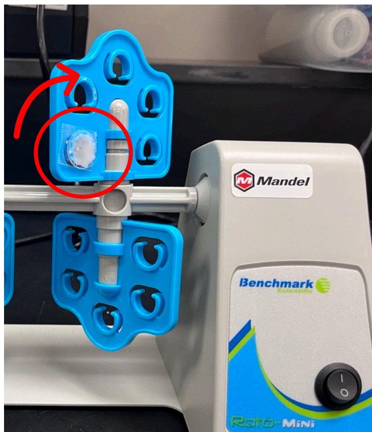
Figure 7. Image of the RotoMini with a glass cover slip attached by double sided tape (circled in red)
