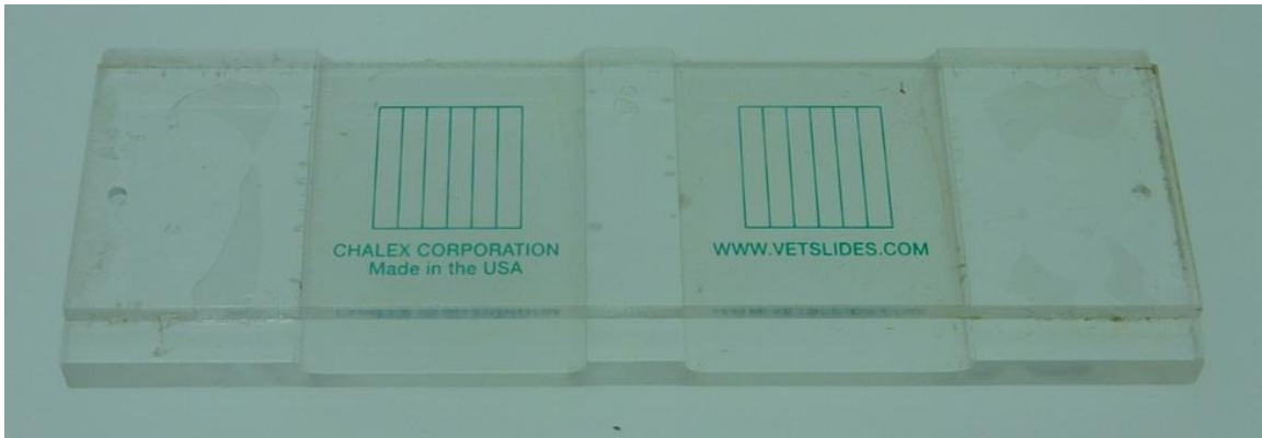
Figure B1. Two-chamber McMaster counting slide used for FEC floatation of ruminant feces (Chalex Corporation, USA).
