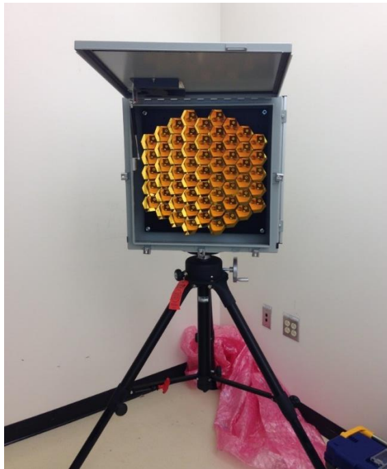
Figure 25 The retroreflector array on a tripod.
