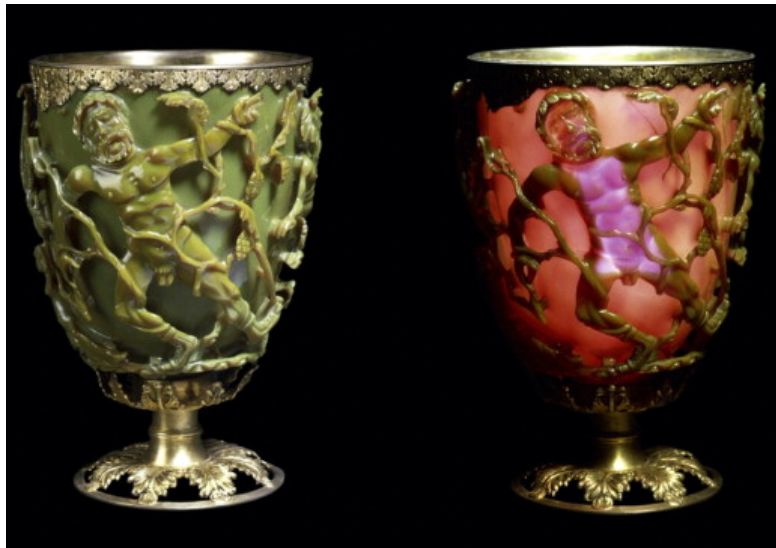
Figure 3: Lycurgus cup example of the interaction of gold and silver nanoparticles with light. 22
