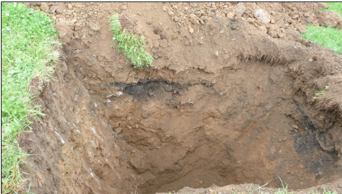
Plate 10: Partial east wall profile of TP-04 showing the dumped asphalt layer.
