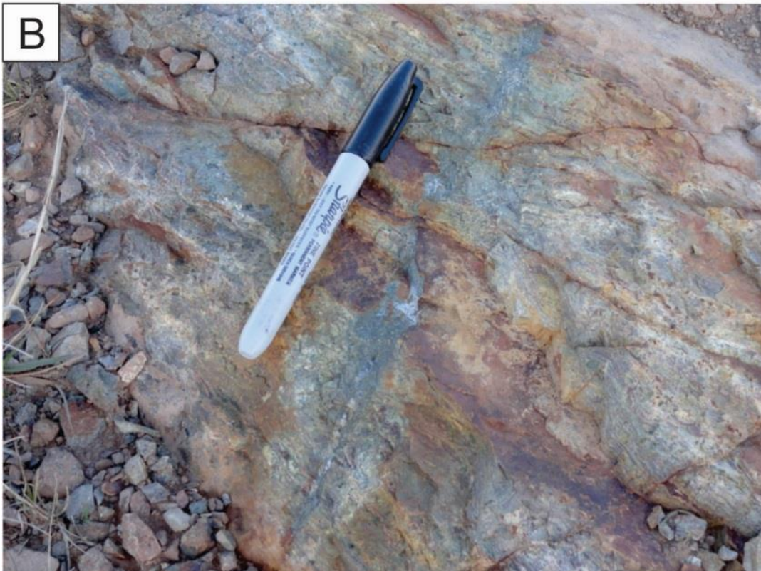
Figure 2 - Outcrop at Warwick and Nuttby Mountain Au occurrences. A) Silicified and sulphidized basalt from Warwick Mountain and Nuttby Mountain outcrops. Assays returned up to 660 ppb gold. B) Sulphide veinlet cross cutting rhyolite. Assays returned up to 150 ppb gold.
