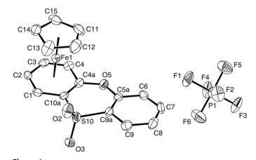
The cation and anion of complex (I), showing the atom-labelling scheme. Displacement ellipsoids are drawn at the 50% probability level. H atoms have been omitted for clarity.
