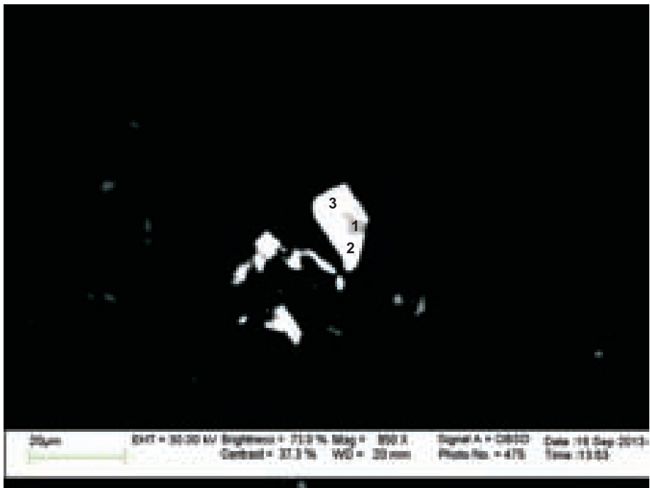
Figure 1-3.9b: Horton group sample 2349B site 22; darker BSE image of figure 9a. Monazite partially replaced(?) by Fe-oxide (analysis 1)
