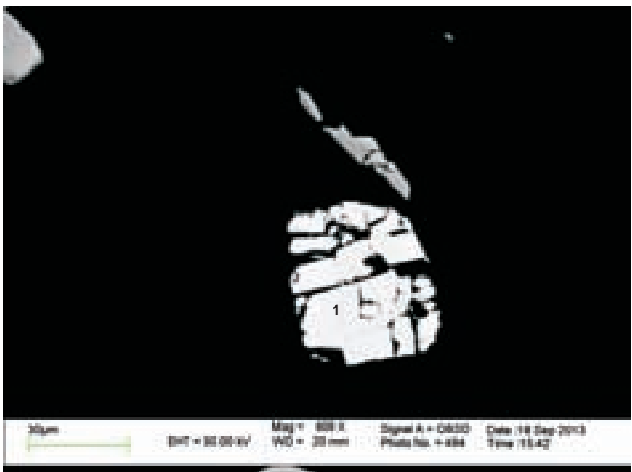
Figure 1-2.7b: Horton group sample 2349A site 19; darker BSE image of figure 7a. Xenotime, unclear whether it is of detrital or hydrothermal origin.
