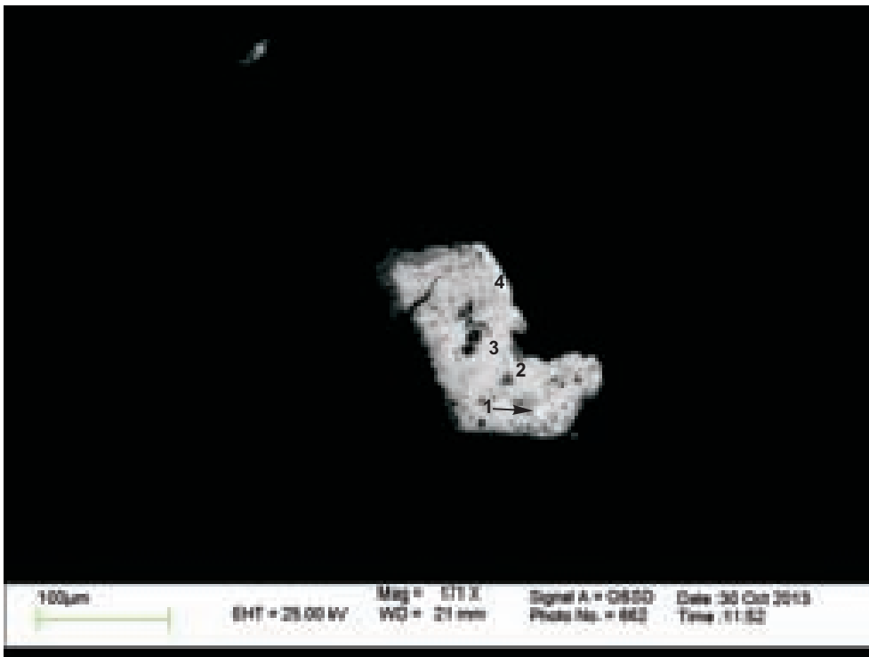
Figure 2-2.12A: Sample 9874 site 11; magmatic zircon with Fe-oxide overgrowth (analyses 1&2), is cut by fracture and contains dissolution voids. Zircon contains Y (~6.5%) and Yb(~1%).
