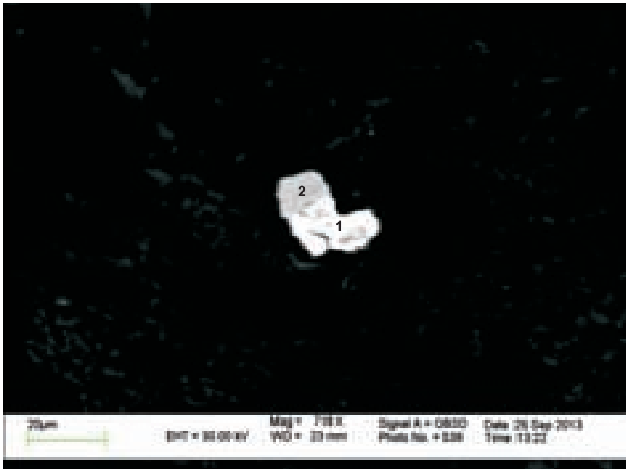
Figure 3-2.6b: Lamprophyre dyke sample C2226 site 6; brighter BSE image of figure 6a. Xenotime appears to replace earlier pyrite.
