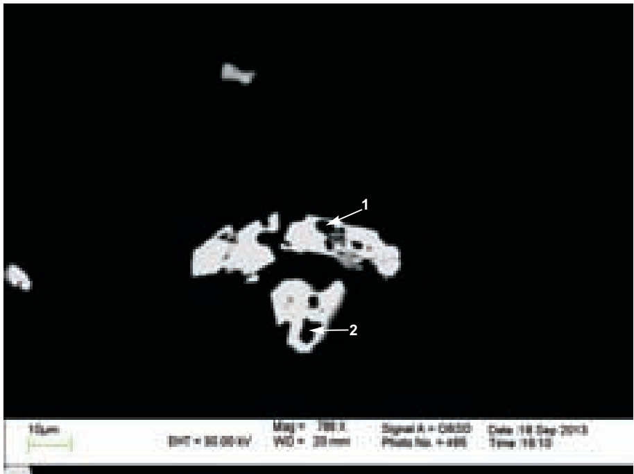
Figure 8b: Horton group sample 2349A site 22; darker BSE image of figure 8a. The monazite crystals contain quartz inclusions.
