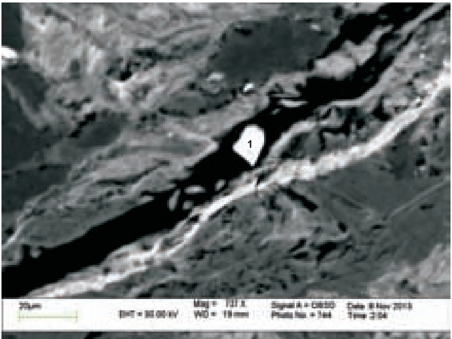
Figure 2-5.56: Sample 9877 site 24; Horton Group. Fragment of Ti-magnetite grain in fracture.
