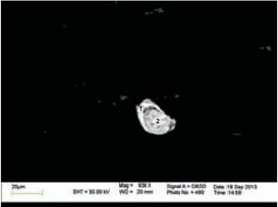
Figure 1-2.5b: Horton group sample 2349A site 14; detrital zircon (analysis 2) enriched in Y, with rim of hydrothermal zircon (analysis 1) with a more pure composition.
