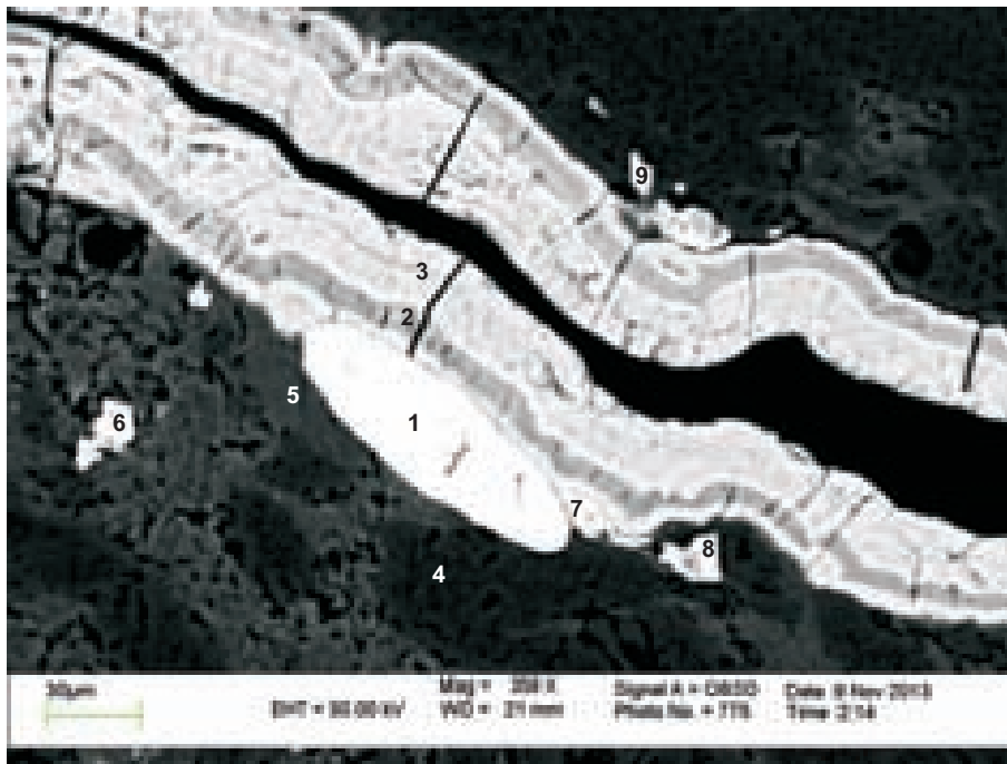
Figure 2-5.44: Sample 9877 site 63; Horton Group. Zircon postdated by later Fe-oxide mixture in fracture with cooling cracks. Fracture filled with successive zones of Fe-oxide and chalcopyrite intermixed with chlorite and phosphate.
