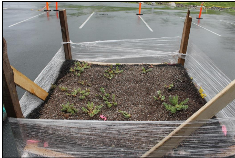
Figure 4: Typical plant cover on native plant mat before installation on the NSCC green roof. Main species before installation was Rhodiola rosea .
