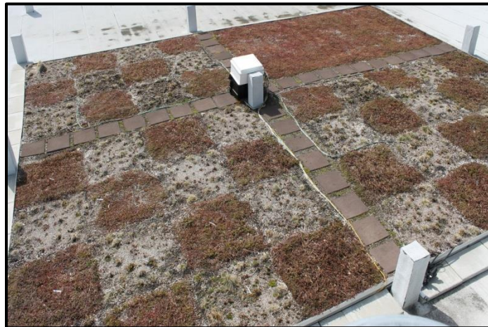
Figure 21: NSCC green roof on April 18, 2014. Dark coloured plots are Sedum , lighter plots are native species.
