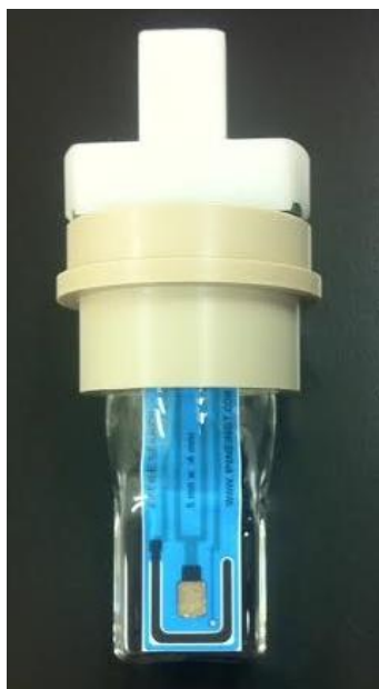
Figure 5. Photo of the setup used for EC-SERS, including the flat-walled vial, AgNP-modified screen printed electrode, and holder for connection to the potentiostat.
