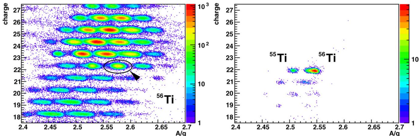
Fig. 1. (Color online.) *Left*: Charge vs. mass-to-charge ratio before the breakup target at the S2 focus of the FRS. *Right*: Charge vs. mass-to-charge ratio of fragments at the S4 focus of the FRS with  $^{56}\text{Ti}$  identified at S2.
