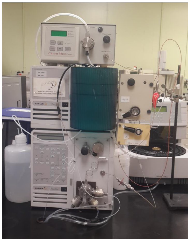
Figure 3.2.4 Online HPLC instrument.
