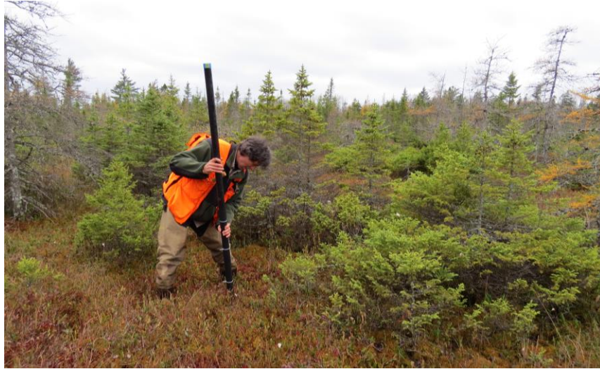
Figure 7. Well installation for a Hobo groundwater-level recording device (Brazner et al. 2015)
