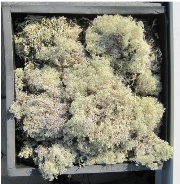
Figure 2. A Cladonia module used in the lichen trial. Each module had a length and width of 36cm with a substrate depth of 6cm.
