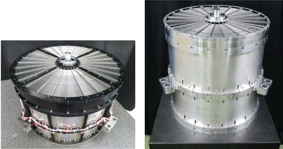
Figure 4. Photographs of flight models of (left) Soft X-ray telescope, SXT-2 and (right) hard X-ray telescope, HXT-1.
