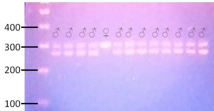
Figure 1. Visualization of IDH sexing locus amplifications. PCR products run out on 2% ethidium bromide stained agarose gel with a 100bp ladder for size reference.
