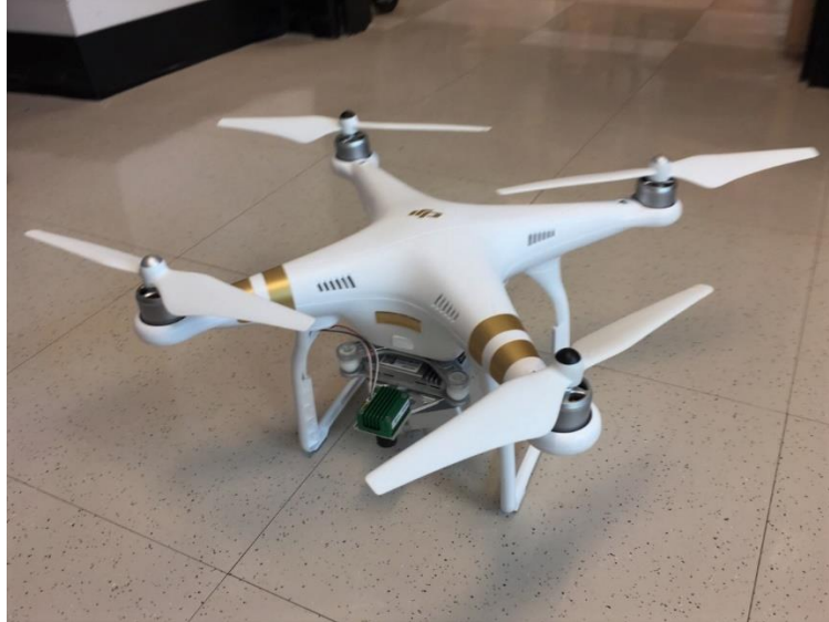
Figure 2.6. DJI Phantom 3 Professional quadcopter used to collect high-resolution multispectral aerial imagery. The aircraft was equipped with a 12-megapixel RGB camera on a rotating gimbal and a fixed Sentera single Near-Infrared sensor.
