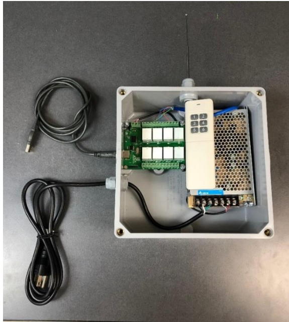
Figure 17: The USB to GPIO board wired to the RF transmitter.
