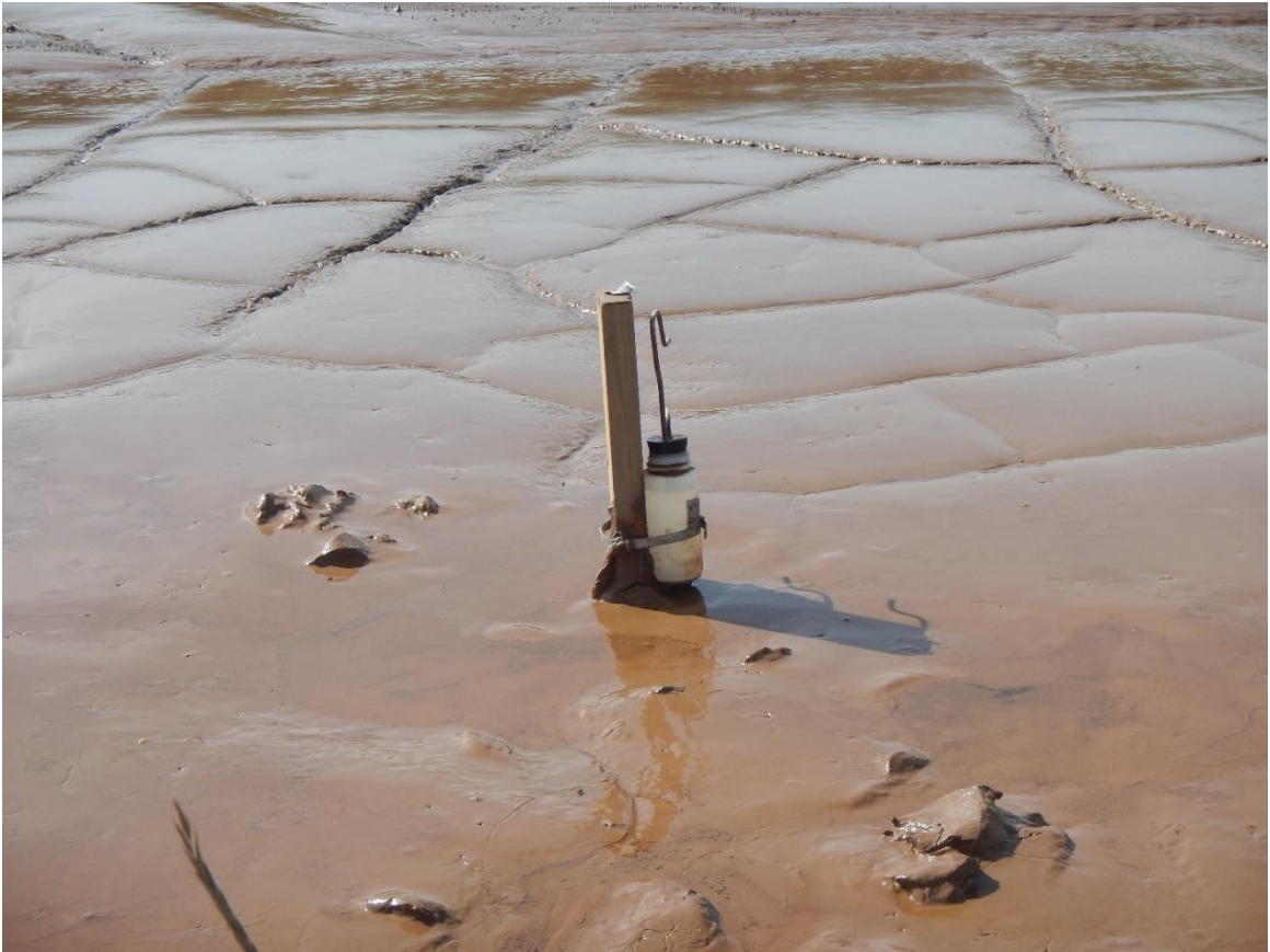
Figure 33: Rising stage bottles installed 20cm above the channel bed were used to measure incoming SSC.
