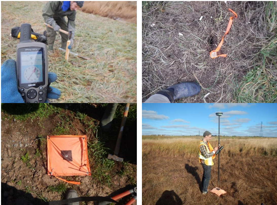
Figure 30: General method for installing GCPs.
