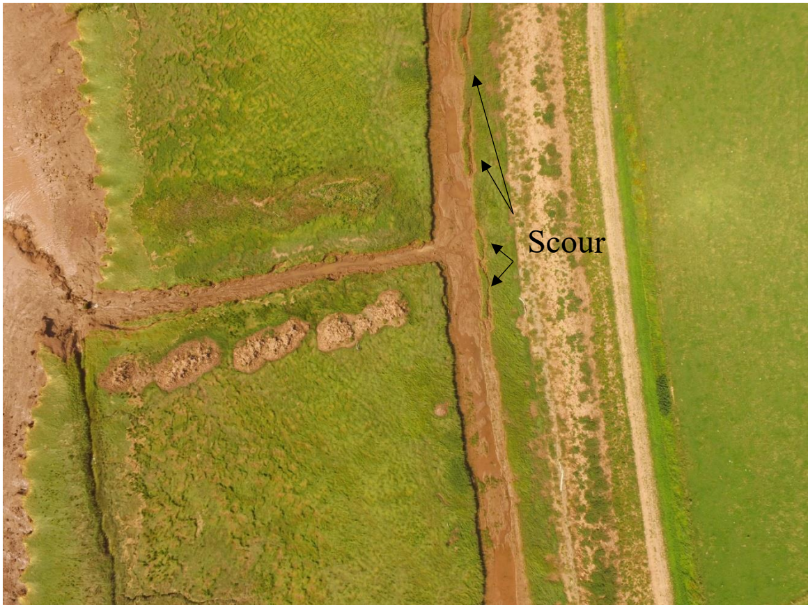
Figure 17: Scouring of backshore saltmarsh caused by the excavation of a borrow pit outlet.
