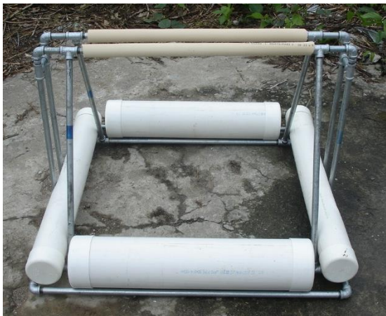
Figure 2: Photo of metal frame (80cm x 80cm) in which C-POD is fixed horizontally.
