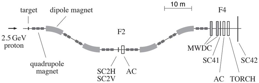
Fig. 1. A schematic view of the experimental setup with the FRS. A carbon target was irradiated with a 2.5 GeV proton beam. The momentum of the deuteron emitted in the  $(p, d)$  reaction was measured by two sets of multi-wire drift chamber (MWDC) at the F4 dispersive focal plane. Scintillation counters (SC2H, SC2V, SC41, SC42) were used for time-of-flight measurements. Čerenkov detectors (AC, TORCH) were installed for confirmation of particle identification.
