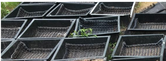
Figure 3. Example of square module with drainage mat barrier included. One module represents one replicate of a particular treatment.
