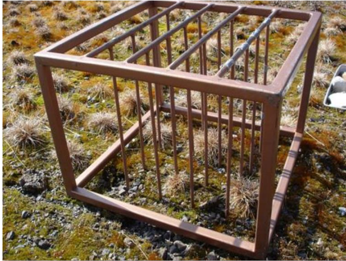
Figure 8. Metal pin frame used for canopy density analysis. The frame contained 16 equally spaced rods which were 6 mm in diameter and rested on the edge of the module. Pins were located approximately 2 cm above the growth medium.
