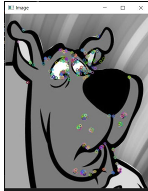
(a) The circular multicolor keypoints in the image are detected using ORB.
