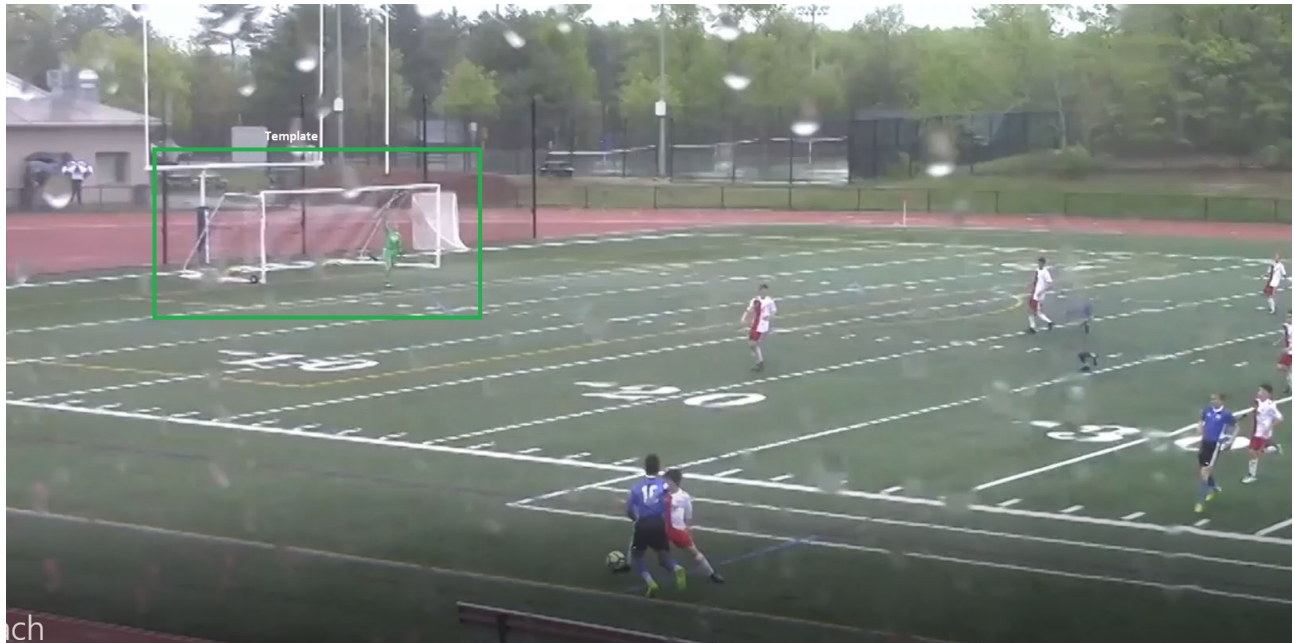
Figure 6.14: The soccer video captured in a football field when it is raining. The rain affects the image quality and the additional white lines of the football field may confuse the matching algorithm. The green rectangular selected area in the image frame is the selected template for the resultant observations.
