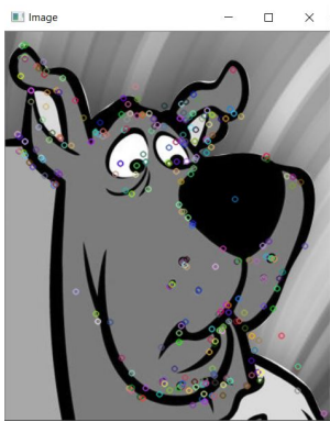
(b) The circular multicolor keypoints in the image are detected using SIFT.
