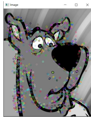
(c) The circular multicolor keypoints in the image are detected using SURF.
