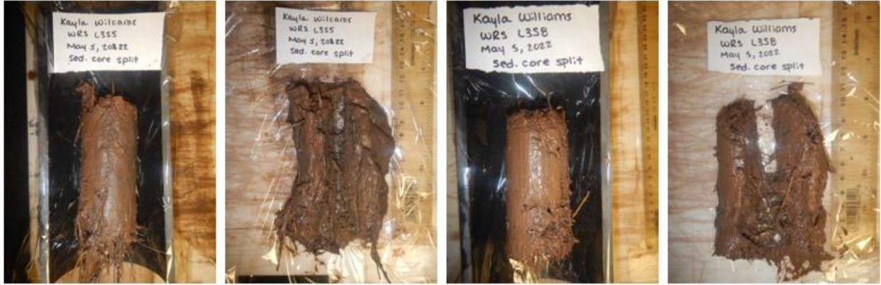
Walton River Reference sediment core and split core sections for samples collected in spring 2022.
