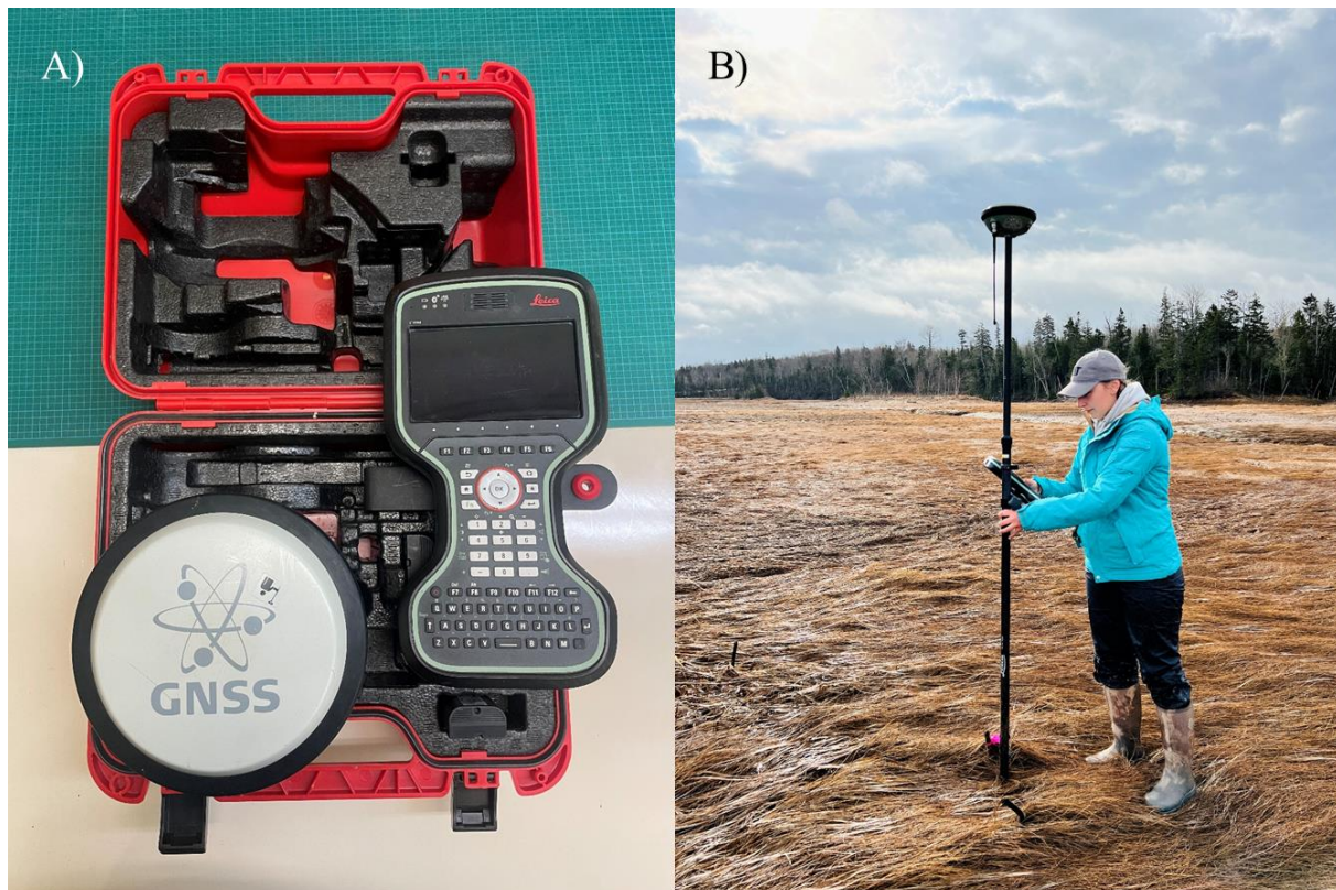
Figure 3.5. A Leica GNSS RTK surveying unit: A) in the case and B) in use (Leica Geosystems; GS14).
