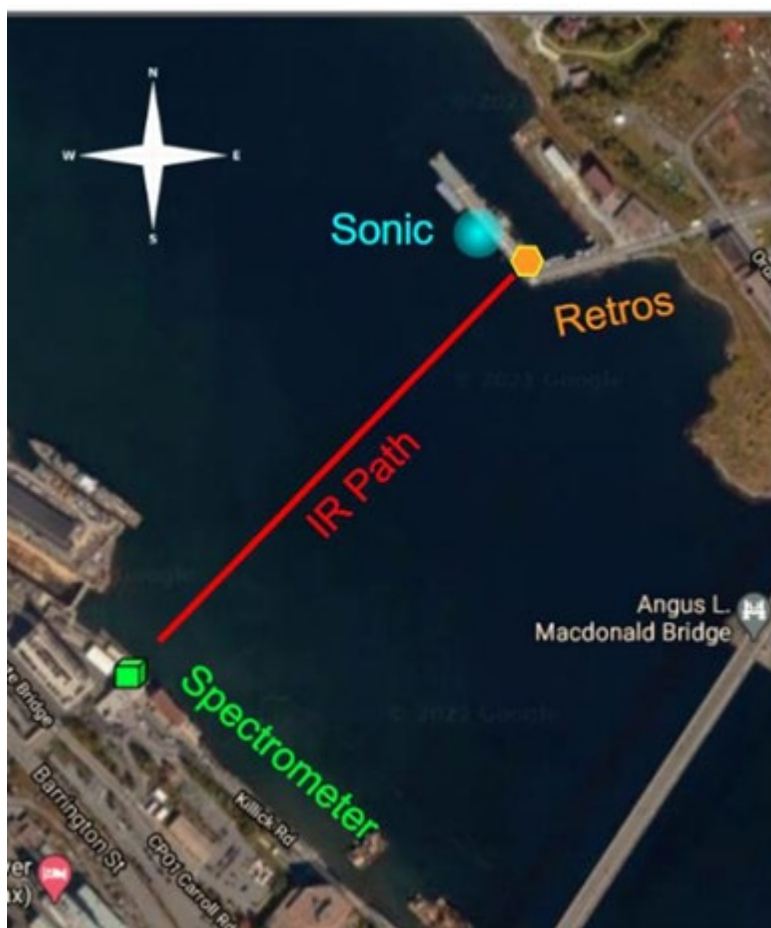
Figure 1-3: Experimental setup. Adapted from Hellmich (2022). Infrared radiation is continuously generated at the spectrometer, traverses the open path to the retroreflectors (alternating continuously between the top height and the bottom height), which reflect it back to the spectrometer, where a detector is co-located and an absorption spectrum is recorded. A 3-D sonic anemometer was deployed outside of the period studied in this work (i.e., from Dec 2020 to May 2021).
