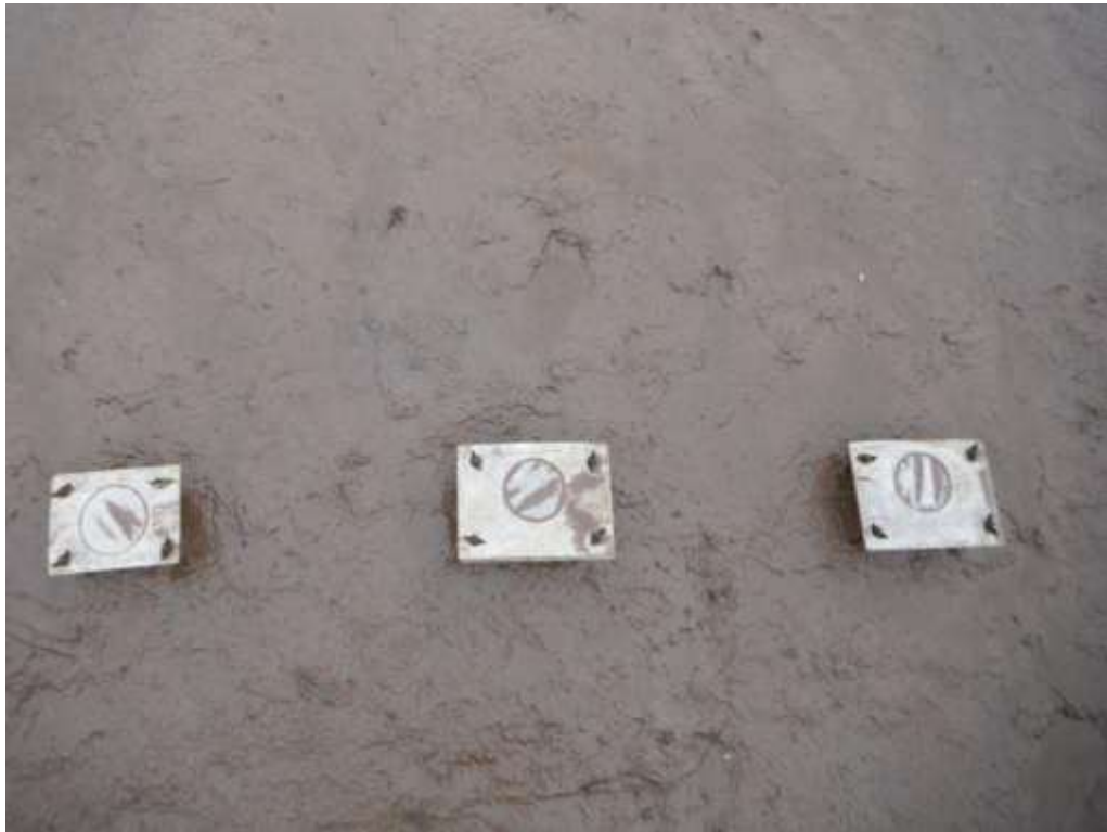
Figure 3.4: Sediment Traps- The method used for capturing deposited sediments.
