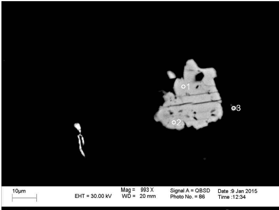
Figure 2-4.11: Sample Newburn 4913.8m site 11 (SEM). Close up of analysis 1 Figure 2-4.10. diagenetic xenotime with fractures.
