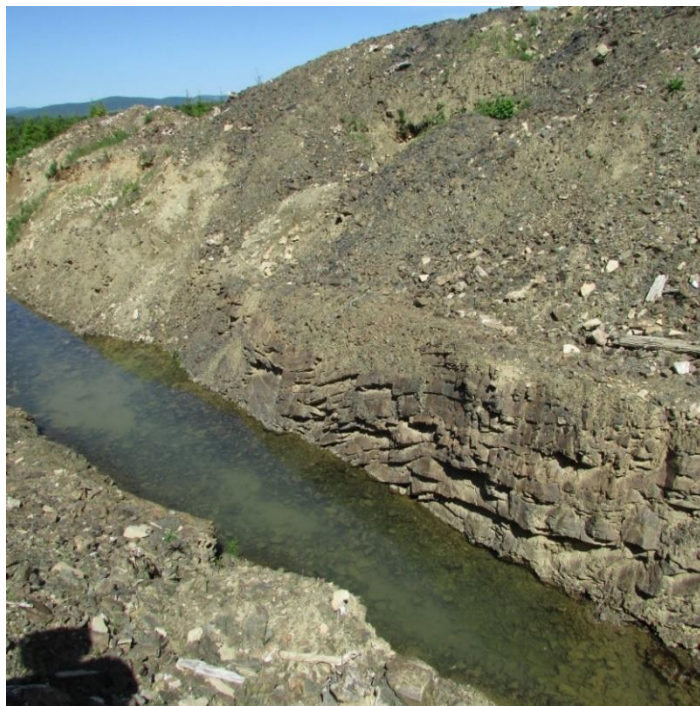
Figure 3 – Maisie trench exposing auriferous quartz vein, northwestern New Brunswick. a) View above trench showing sediment and sedimentary rock overburden, with person for scale. b) View of walls and bottom of trenched quartz vein showing fragments of loose quartz vein material, and folded/ layered host rocks.
