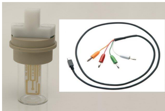
Figure 2.2: The setup used for EC-SERS, including the flat-walled vial, AuNP-modified screen printed electrode, and holder for connection to the potentiostat
