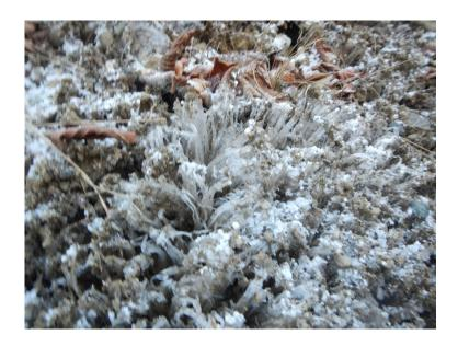
Figure 17) Example of sediment on top of ice crystal formation on the surface of exposed soil in Plant treatment taken November 30, 2015.
