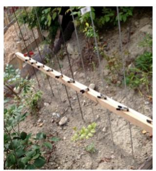
Figure 1) Measuring soil surface position in a Plant treatment plot using profile gauge.
