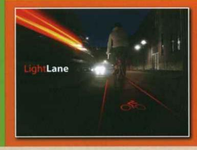
DIY SAFETY. The LightLane is an ingenious idea to make night bike riding safer. Lasers mounted on the rear of the bike project sharp, bright lines onto the pavement behind the cyclist, creating a virtual and movable bike lane, complete with a cycling logo. This gives drivers a boundary and keeps cyclists out of harm's way. Creators Evan Gant and Alex Tee of Boston presented their idea in an online design contest. They are now working on a prototype, (Courtesy Evan Gent, Altitude Inc.)
