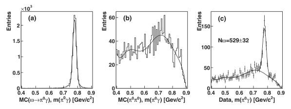
FIG. 3. Same as Fig. 1, but for  $E_{\gamma}=1325$  MeV. A Gaussian fit to the  $\omega$  peak results in  $\sigma=13.6$  MeV (FWHM = 32.0 MeV). A polynomial of order eight used to fit the background.
