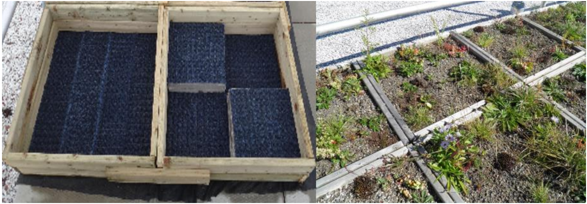
Figure 4.1. Experiment before and after planting. The image on the left shows the homogenous 15 cm treatment (left planter box) adjacent to the heterogenous 5/15 cm treatment (right planter box). The image on the right shows the community composition at the end of the first growing season, August 2018.
