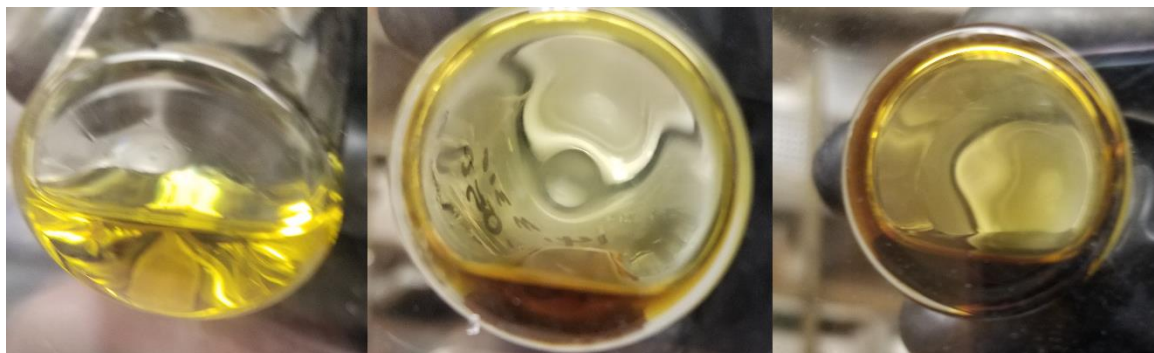
Figure 3.1 Images of B3a (gold, left), B5a (golden brown, middle), and B6a (brown, right) crude reaction mixtures of \text{MoO}_3 and ethylene glycol after heating, concentration in vacuo, and filtration through diatomaceous earth.
