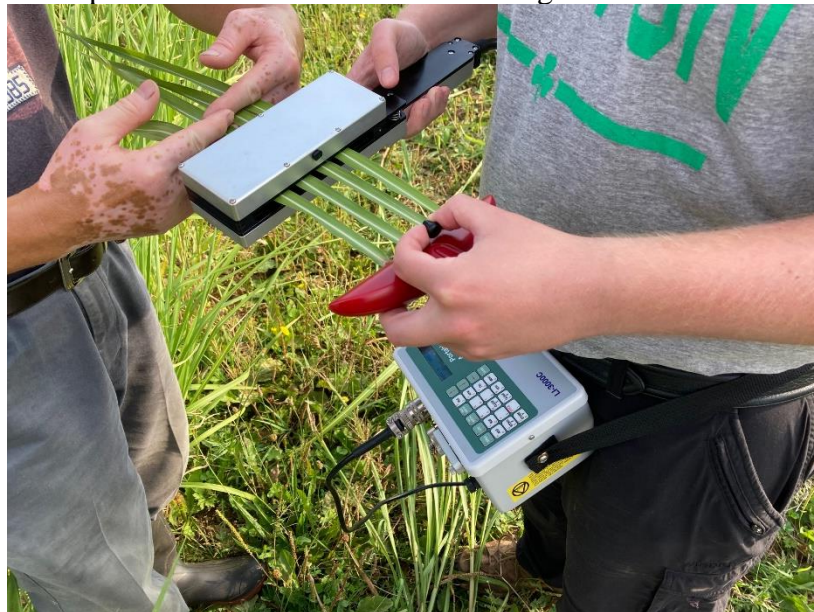
Figure 3.14. Method used to measure multiple Miscanthus blades using the leaf area meter.
